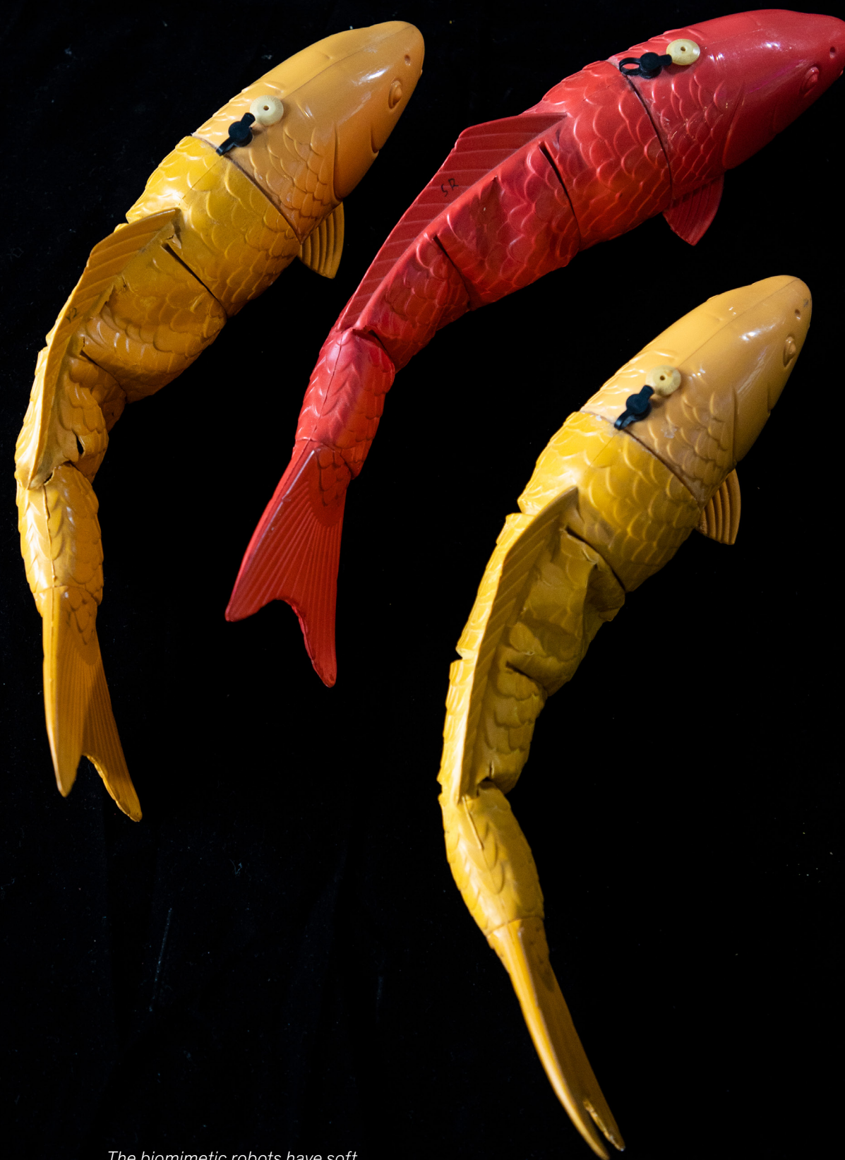
The biomimetic robots have soft fins and swim in an undulating motion.
